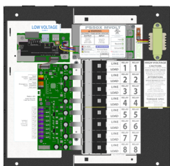
Dead-Front removed Shown with optional voltage barrier and 347VAC transformer
